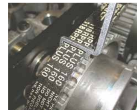
As long as the width of the timing belt does not exceed the width of the timing belt checking tool gauge, the timing belt condition is OK
