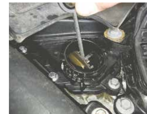
The timing belt checking tool gauge is guided down towards the timing belt through the oil filling hole
