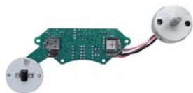
3018 Circuit board for K4213-2
