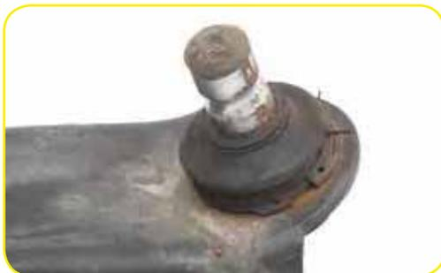
*Here is an example of a loose ball joint, where replacement of a complete track control arm is required*
