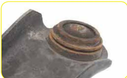
Depending on car brand and model, the replacement of worn/defective ball joints can be a costly affair. The repair costs depend on, amongst other things, whether a complete replacement of the track control arm must be done or if replacing the ball joint and possibly the bushes is sufficient. Although ball joints often are available separately, it is not always sufficient to only replace the ball joint. In the following paragraphs, you will find out why this is – and what you should be aware of.
