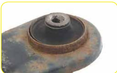
*Here is an example of a worn bushing. In some cases, a replacement of the bushing will be sufficient*
