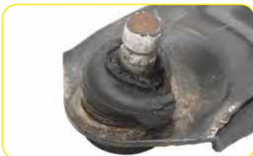
*Here is an example of a damaged ball joint boot. In some cases, a replacement of the boot or ball joint will be sufficient*
