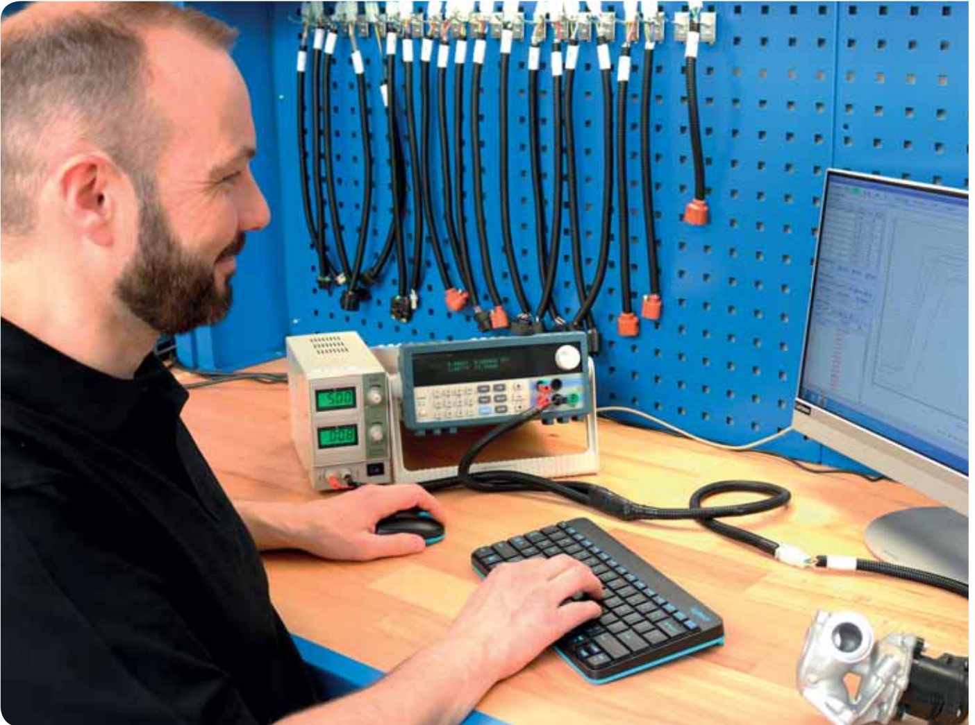
Product Coordinator Lars Berthelsen with the new EGR valve test equipment
