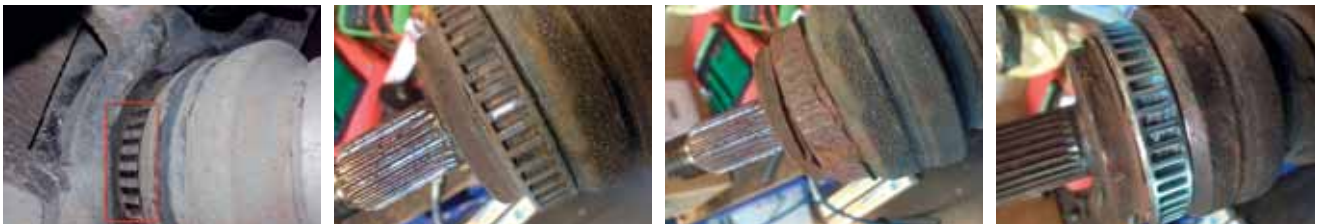
Pictures of drive shaft with a defect and a functional ABS-ring (Autodata)
