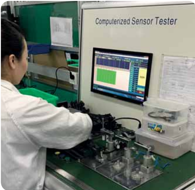
Each Triscan sensor undergoes a 100% quality control
