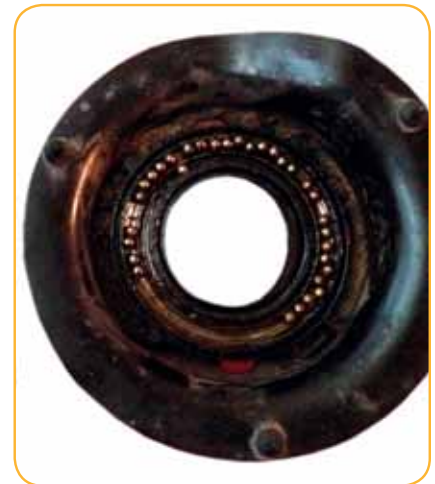
Examples of defective strut mount rings
