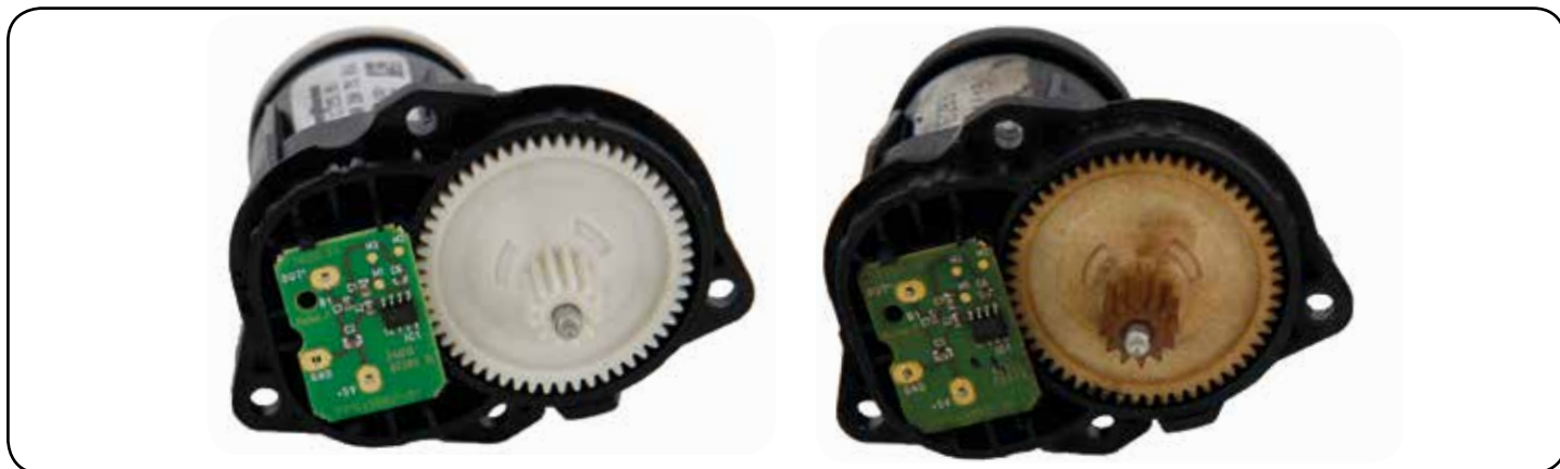
In this picture you can see clearly how the permeated exhaust fumes have sooted the circuit board and its components.
