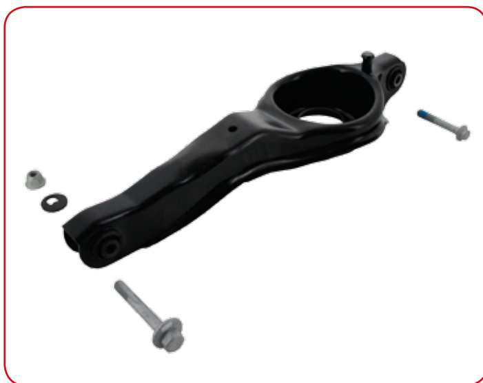
Track control arm with the correct position of the bolts
