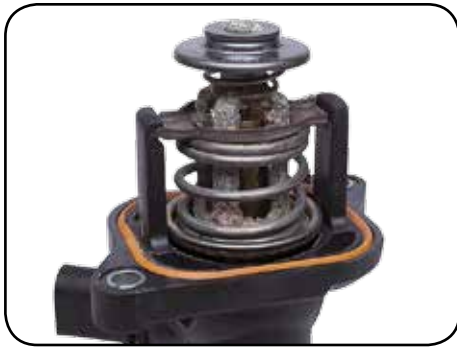
Figure 1 MAP controlled thermostat with clear signs of corrosion (Photo credit: Mahle)
