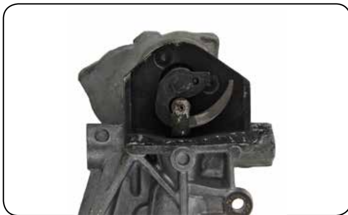
The image clearly shows how the exhaust gas has penetrated and melanised the chamber and the parts included in the valve control mechanism
