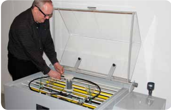
Triscans new salt spray chamber - for accelerated lifetime testing of corrosion protection
