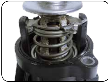
Figure 2 Thermostat with coolant/additive not approved by the manufacturer. This has led to that the aluminum is “etched” away (Photo credit: Mahle)
