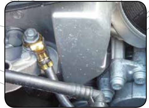
Figure 3 You should check that the ground cable is intact and properly connected (Photo credit: Mahle)
