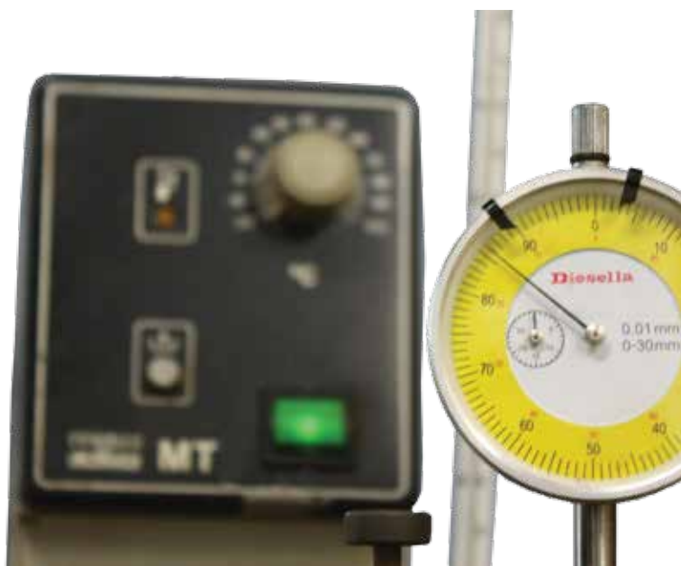
When boil-testing, you place the thermostat in water, which you bring up to its boiling point - it will clearly show if the thermostat opens and closes as it is supposed to
