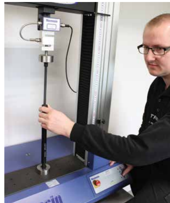
Triscan’s equipment for tensile and pressure testing is, like the ozone chamber, used to test a variety of product lines
