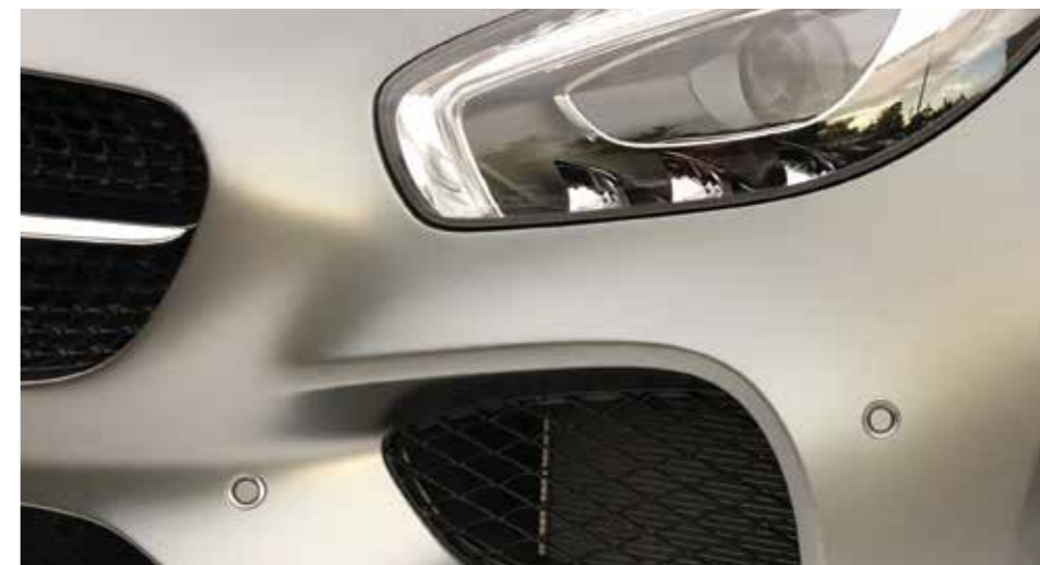
Triscan's programme of vehicle-specific sensors exclusively includes sensors for ultrasonic systems
